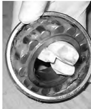
Fig. 10. Grease can easily be packed by hand.
