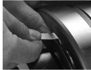
Fig. D-3. Measure RIC before installation.
